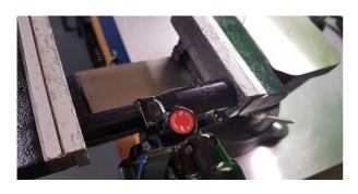
Place the tapered part of the busing tool on the opposite side and carefully place the tool within the vice ensuring the tool is seated squarely.
