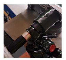
If your replacement bushing is metal rather than a polymer then grease the bushing lightly. Polymer bushings should not be greased. Now with the tapered end facing outwards slowly and gently tighten your vice until it comes to a stop.
